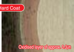
[Oxidisation Evaluation] (Scratches from calotest performed after one-hour exposure to the air of 1,100°C)
