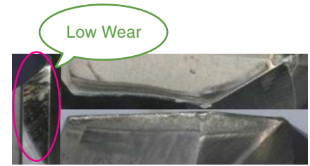
Cutting Conditions : f=0.60 mm/rev Cutting Length : 60m Cutting Time (39min)
