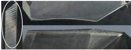
Cutting Conditions : f=0.30 mm/rev Cutting Length : 30m Cutting Time (39min)
